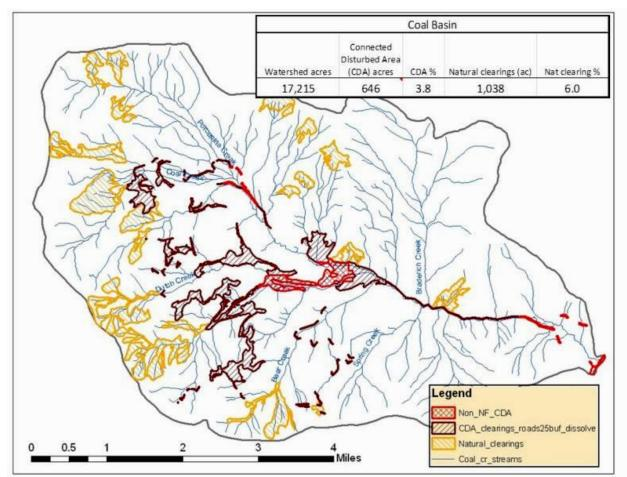
Figure 12. Connected Disturbed Areas in Coal Basin (Source: WRNF).
