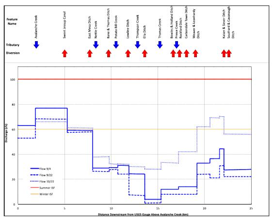
Figure 5. Longitudinal flow profiles, Lower Crystal River 2012. This figure plotted longitudinal changes in streamflow under the assumption that changes in discharge occur at discrete locations where the river experiences tributary inflows or diversions.
