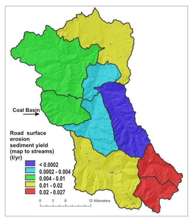
Figure 21. A HUC 12 basin classification of predicted and basin-averaged road surface erosion rates reveal that the southeast subbasins – the North Fork and South Fork Crystal River subbasins - have the highest average road erosion values across the Crystal River watershed.
