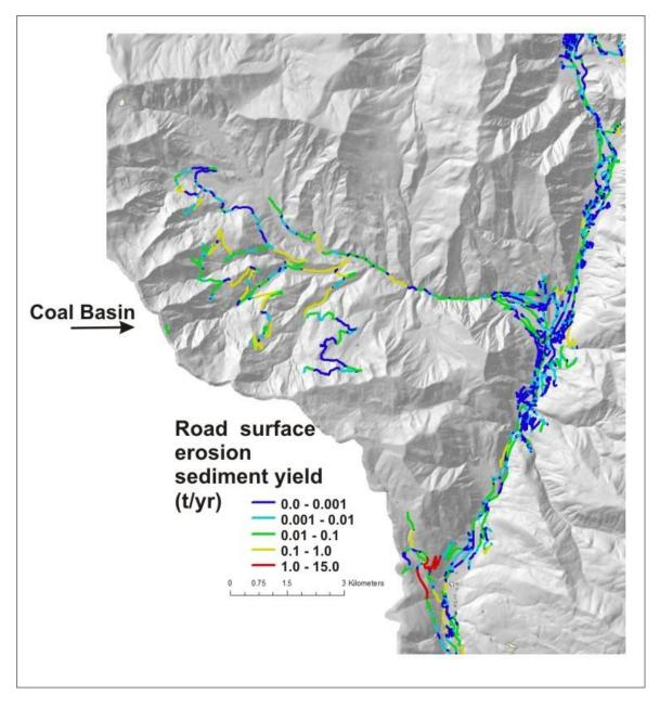
Figure 20. NetMap WEPP: Road was used to calculate road surface erosion per road segment. The focus is on Coal basin within the Crystal River basin where several road segments yield above 0.1 t/yr.
