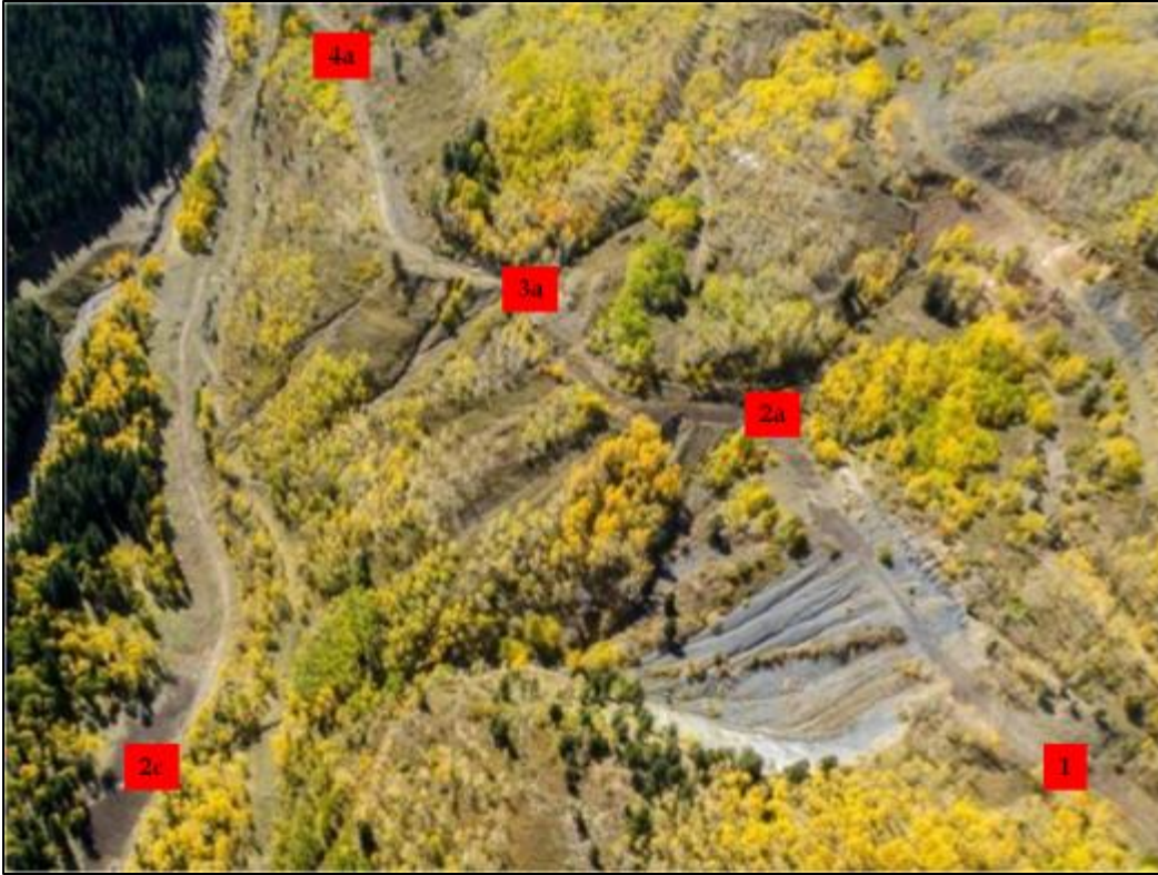
Figure 5. Pilot project area with work ongoing, September, 2012 (source: EcoFlight). Note the darkened surface at area 2c (“alluvial fan”) area, where the largest volume of compost/biochar was applied.
