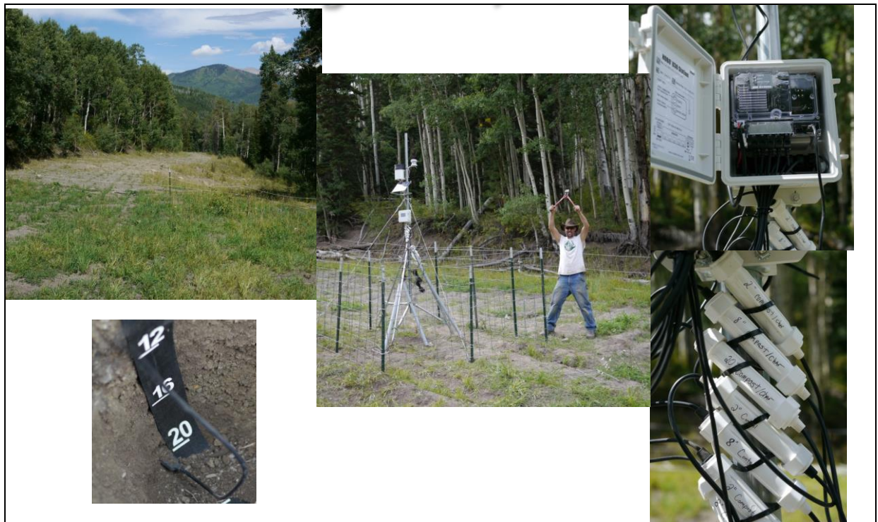
Figure 22. Soil moisture monitoring station. August 2013.
