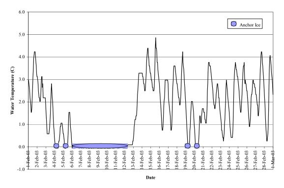
Figure 13. Hourly water temperatures during February 2003 at Palm Site.
