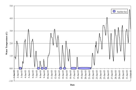
Figure 12. Hourly water temperatures during January 2003 at Palm Site.
