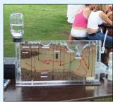
Materials: lexan, sand, gravel, plastic tubing, water **Purpose:** demonstrate how water moves underground and is affected by pumping
