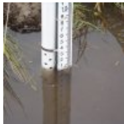
Photo 4.2: Water depth gauge, Courtesy of WWMMP.
