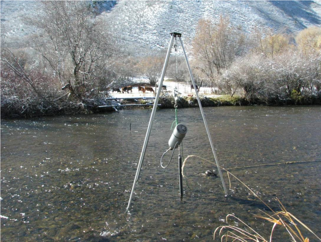
Figure 2. Freeze core apparatus.
