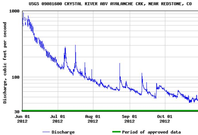
Figure 4. Crystal River hydrograph for the summer and fall of 2012. Y-axis ranges from 30 to 1,000 cfs. Noteworthy are the significant spikes in flow from summer monsoonal events.
