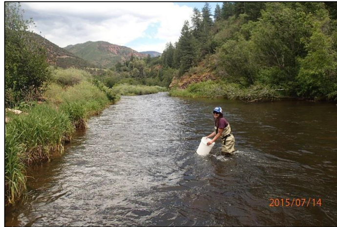
Figure 1. Colorado Mountain College field technicians observing didymo coverage with a gridded viewing bucket
